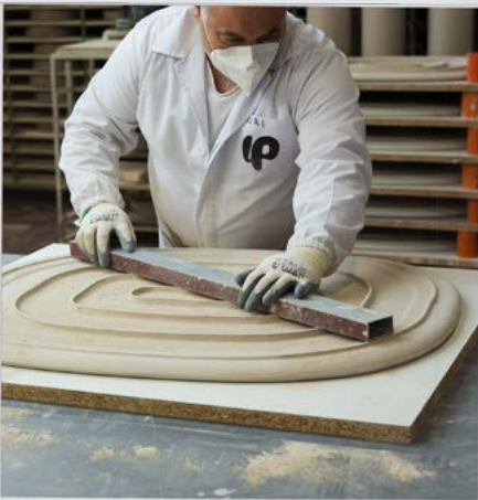
After drying, the tabletop is smoothed by hand
